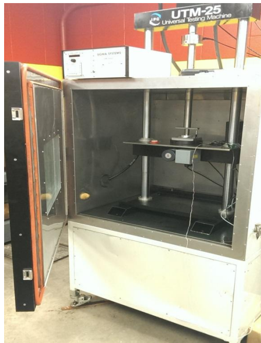
Figure 5-1 : Servo-hydraulic testing machine UTM – 25.
